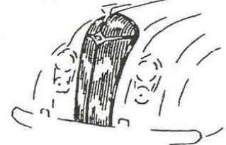
The last of the Airflows changed hood and grille completely, but retained identical front quarters. The hood opens at the belt line instead of from bumper level, and the grille follows the styling trend of the rest of the 1937 Chrysler line, being again light weight stampings with stainless steel trim.
